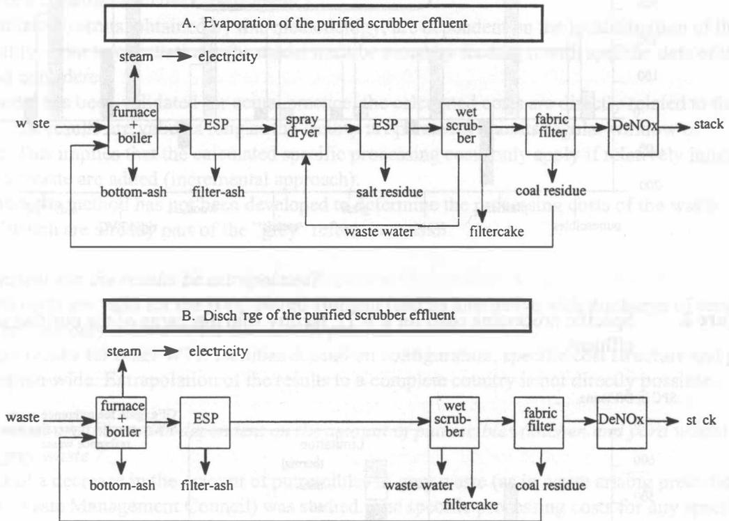
**Figure A.1** Process configurations considered in this study.
