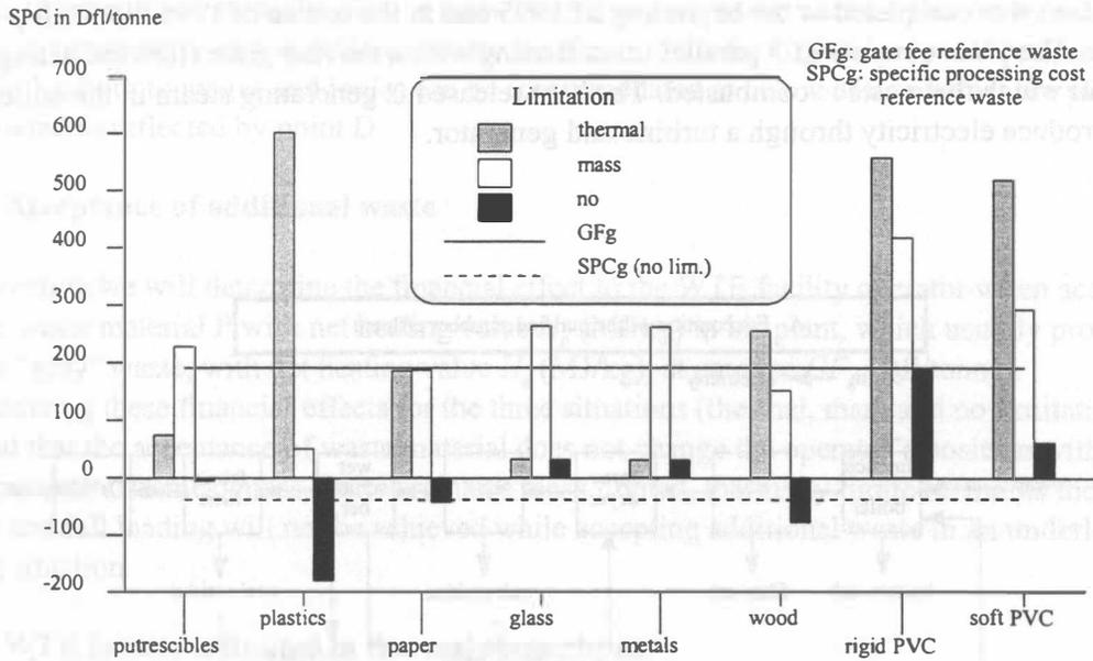
**Figure 2.** Specific processing costs for a WTE facility with discharge of the purified scrubber effluent.
